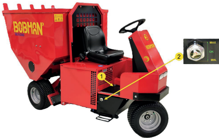
(1) Hydraulic oil tank plug / (2) Oil level indicator
